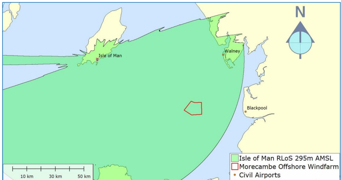
Figure 15: Isle of Man RLoS 295m AMSL
